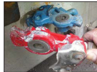
Powder Coated - corrosion has begun where the coating has chipped
