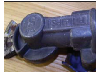
Anodized - Virtually no corrosion on the body
