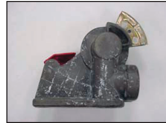
Anodized - minimal corrosion where scored
