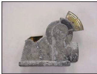
Standard - Heavy corrosion on entire body
