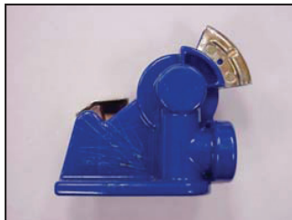
Powder Coated - Minimal corrosion where scored
